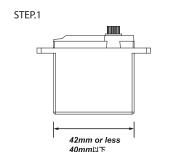
Use a servo with a width of 40mm or less.
