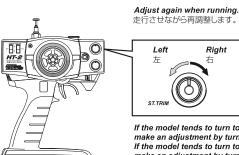
If the model tends to turn to the right, make an adjustment by turning the trim to the left. If the model tends to turn to the left, make an adjustment by turning the trim to the right.
