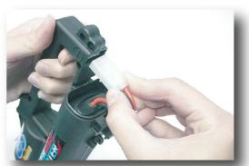
M: Install an AA size battery into the glow igniter as shown. Replace the spring and end cap and tighten fully. After usage, always remove the battery from the igniter. More powerful aftermarket rechargeable igniters are available at your local hobby shop.
