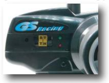
I: Now check the neutral 'trim' settings. With the steering wheel and trigger in the neutral position (hands off), the wheels should be pointing straight ahead, and the throttle servo horn should be pointing straight back and forth with the carburetor in the neutral (closed) position. If either servo is not centered, rotate the steering and throttle trim knobs accordingly to place both servos in the correct neutral position.
