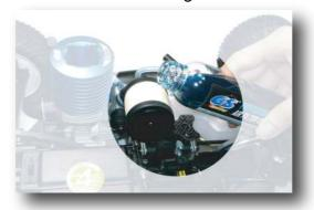
K: Fill your fuel bottle with brand name 20% model car glow fuel. Lift the lid of the fuel tank, place the tube of the fuel bottle over the opening, and full with fuel. Be careful not to spill fuel
