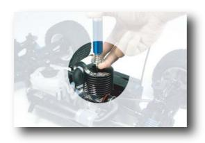
Q: After the engine has broken in and tuned for proper speeds and performance, you will likely need to fine tune between race weekends or even on the same day. Adjust only one needle at a time, and in one hour increments.
