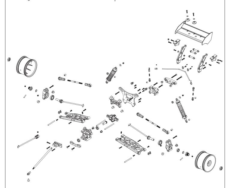
**Rear Lower Arms:** Thread a 4x10mm set screw through the hole on the tab of the inside of the right and left arms until it sticks out 1.5mm. You will recheck this down stop setting later.
