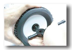
C: Check the tires to make sure they are fully glued to the wheels. Gently peel the tire away from the wheel, and if you find any spots where there is a gap between the tire and wheel, apply a small amount of CA glue.
