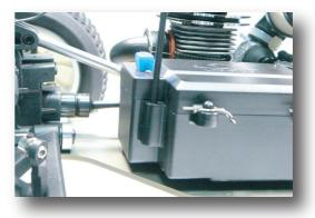
F: Remove the radio box cover by removing the small clip and lifting the cover out. Remove the battery tray from the box and install four AA size batteries. Again, always use fresh, fully charged batteries. Place the battery tray back in the box and replace the cover and clip.
