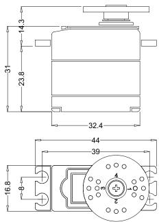
2.FEATURES 3-POLE FERRITE MOTOR LONG LIFE POTENTIOMETER 1-OILITE BUSHING AND 1-BALL BEARING INDIRECT POTENTIOMETER DRIVE HYBRID I.C
