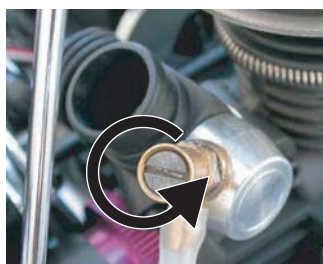
(D) Rough at full throttle: Turn needle 1/4 turn counter clockwise. (open) Continue 1/4 turn increments until full throttle is smooth and responsive.
