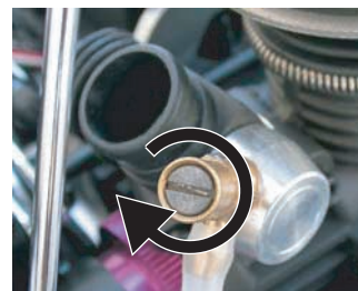
(B) After the first tank of running the truck, turn needle valve 1/4 turn clockwise (closed). Then follow the same step on next three tanks. So after the 4 tanks of running the truck your needle setting should be 3 turns from fully closed.
