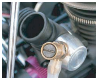
(A) Needle Valve Starting Position: Turn needle valve clockwise until it stops. (closed) Open counterclockwise 4 turns. (open)
