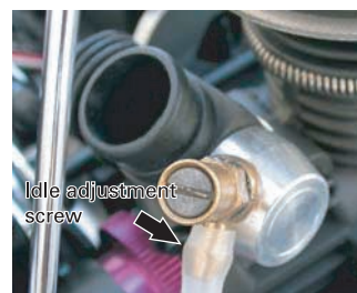
(E) Adjusting idle: Turning clockwise increases idle RPM. Turning counterclockwise decreases idle RPM.
