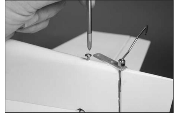
□ 25. Place 2–3 drops of thin CA in each hole to harden the surrounding wood. Doing so will make the screws more secure, preventing them from vibrating loose.
