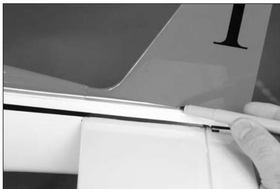
3. Remove the fin from the fuselage. Use a straight edge and hobby knife with a new #11 blade to trim the covering 1/16-inch (1.5mm) below the line on the fin to expose the underlying wood.
