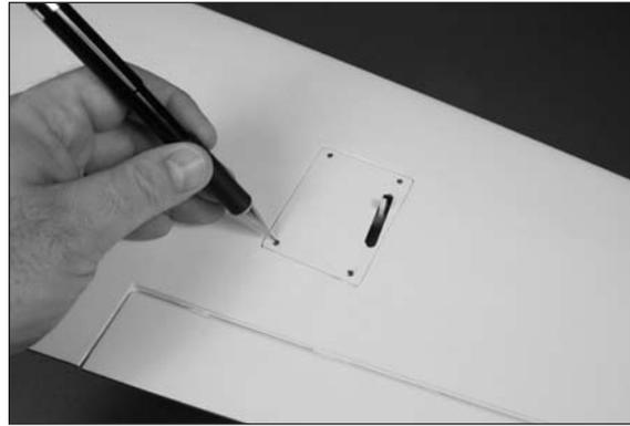
□□ 19. Remove the cover and servo from the wing. Use a pin vise and 1/16-inch (1.5mm) drill bit to drill the four holes for the cover mounting screws. Make sure not to accidentally drill through the top of the wing.
