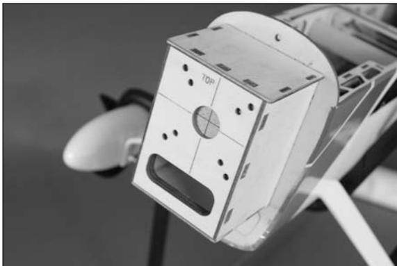
□ 2. Use a drill and 1/8-inch (3mm) drill bit to drill the four holes for mounting the engine. Use the inner set of holes for the Power 25, the outer set of holes for the Power 32.
