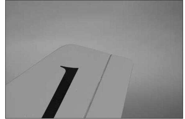
□ 19. Saturate each hinge using thin CA on both the top and bottom of the hinge. Allow the CA to fully cure before proceeding.
