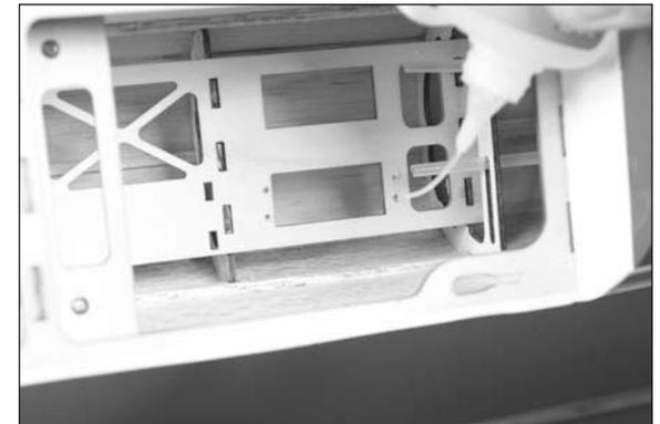
□□ 8. Secure the elevator servo in the fuselage using the screws provided with the servo and a #1 Phillips screwdriver. Make sure the output of the servo faces to the rear when installed in the fuselage. Route the servo lead through the servo tray in the location shown in the photo.
