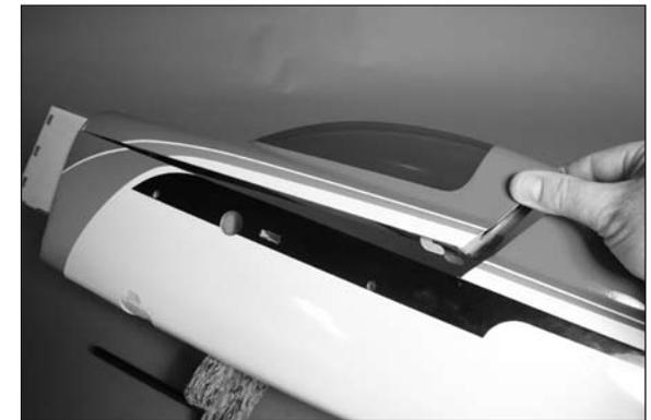
□ 4. Locate the carbon wing tube. Slide the tube into one of the wing panels. It will slide in easily, so do not force it further than it will easily slide.
