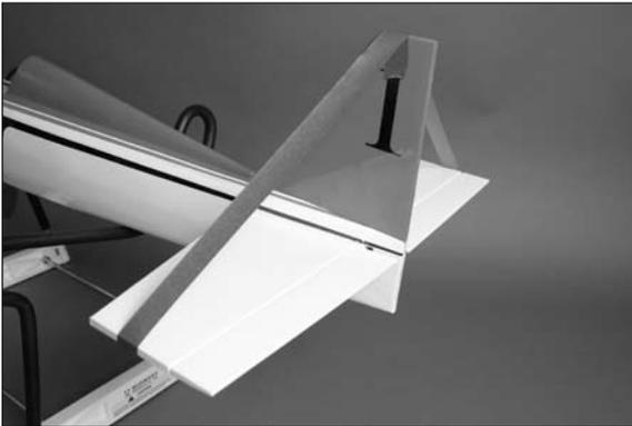
□ 8. Use a pin vise and 1/16-inch (1.5mm) drill bit to drill a hole that is 1/2-inch (13mm) deep 7/8-inch (22mm) from the bottom of the rudder.
