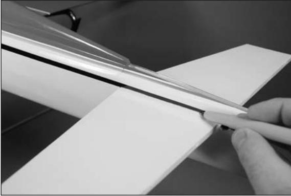
□ 11. Remove the stabilizer from the fuselage. Note the direction of the top and bottom of the stabilizer indicated by the tape placed on it back in step 1. Slide the elevator into the slot, noting the top and bottom to match that of the stabilizer that was just removed.
