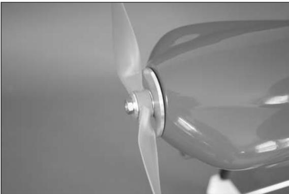
**Important:** Always balance the propeller before securing it to the motor. An unbalanced propeller can transmit vibrations into the motor or airframe, causing damage or even failure of these components.
