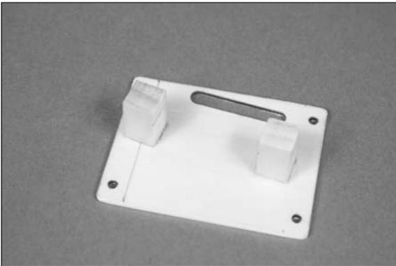
□□ 12. Test fit the servo cover in the opening in the wing. It may be necessary to notch the cover support rail to clear the hardwood block. Use a rotary tool and sanding drum to carefully notch the rail, being careful not to sand the wing sheeting or remove too much material from the rail.
