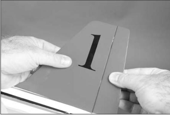
□ 21. Flex the rudder through its range of motion a number of times to break in the hinges. This will reduce the load on the servo for those first flights.
