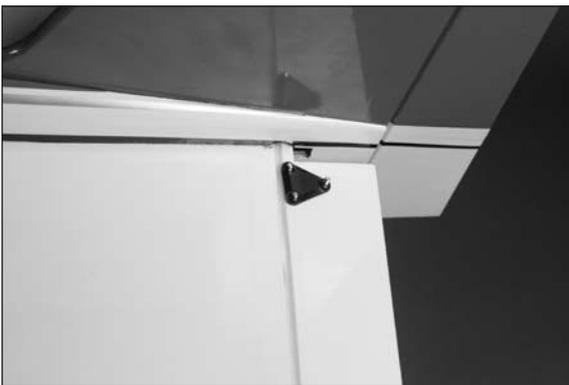
□□ 16. With the elevator servo centered, thread the nylon clevis on the pushrod wire. When the clevis is attached, the control surface must be centered as shown.
