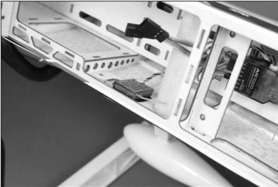
4. Secure the battery in the fuselage using hook and loop straps. Use a piece of hook and loop tape along the bottom of the battery to keep it from sliding on the battery tray.
