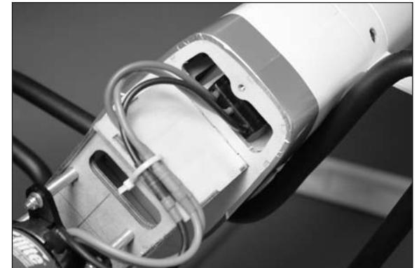
**Note:** Drill a 1/8-inch (3mm) hole in the bottom of the motor box and use a tie wrap (not included) to secure the wires so they don't interfere with the operation of the motor.
