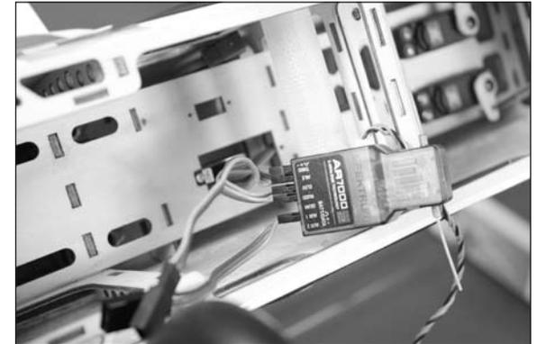
2. Use hook and loop tape to secure the receiver in the fuselage. Make sure to route the leads so they don't interfere with the operation of the servos.
