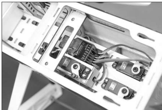
□ 4. Mount the remote receiver in the fuselage away from the main receiver using hook and loop tape. Make sure to orient the antenna on the remote receiver in a different direction than those on the main receiver for the best reception from your radio system.
