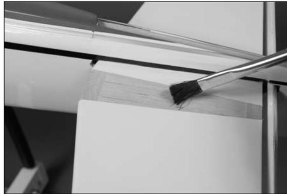
□ 14. Slide the stabilizer in position. Use a paper towel and rubbing alcohol to remove any epoxy that oozes out when the stabilizer is positioned.
