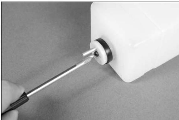
□ 10. Slide the fuel tubing (not included) on the aluminum tubes outside the tank.
