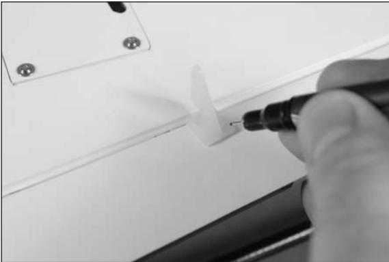
□□ 3. Use a pin vise and a 5/64-inch (2mm) drill bit to drill the holes for the control horn mounting screws.
