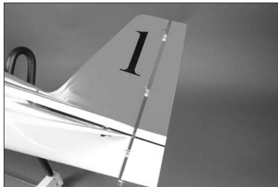
□ 18. Remove the T-pins from the hinges. Make sure the rudder is pressed tightly against the fin to eliminate any hinge gap. Check that the tips of the rudder and fin are aligned.
