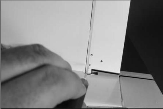
□□ 15. Use a #1 Phillips screwdriver to secure the control horn to the elevator using three 2mm x 12mm machine screws and a control horn backplate.
