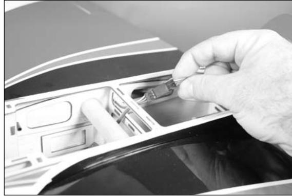
□ 6. Use two 3mm x 10mm socket head screws and two 3mm washers to secure the wings to the fuselage. Use a 2.5mm hex wrench to tighten the bolts securing the wing.
