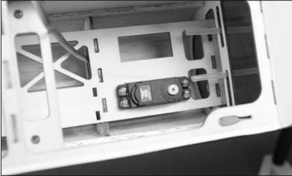
□□ 9. Prepare the servo horn by enlarging the hole in the arm that is 3/8-inch (9.5mm) from the center of the servo horn using a pin vise and 5/64-inch (2mm) drill bit. Use side cutters to remove any other arms from the horn so they don't interfere with the operation of the servo.
