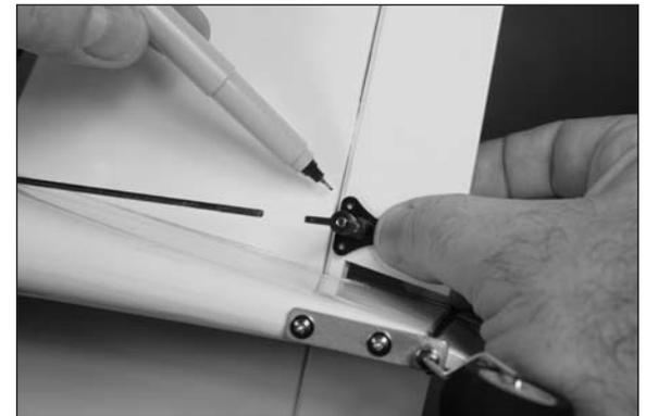
□□ 14. Use a pin vise and 5/64-inch (2mm) drill bit to drill the three holes for the control horn mounting screws. Apply 2–3 drops of thin CA in each hole to harden the surrounding wood.
