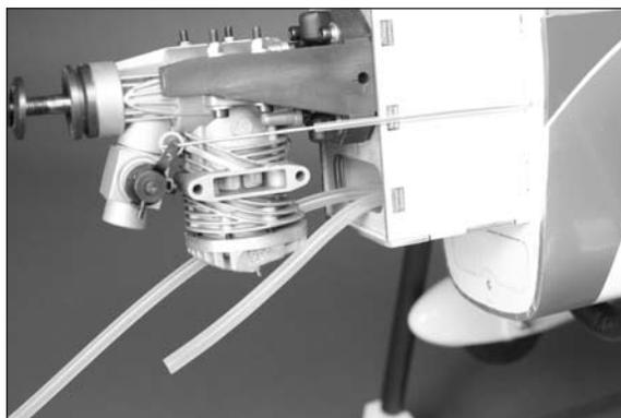
□ 12. Use a razor saw to cut two mixing sticks to a length of 3 inches (76mm). Use these and medium CA to secure the tank in the fuselage.
