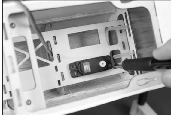
□□ 5. Remove the servo from the fuselage. Use a pin vise and 1/16-inch (1.5mm) drill bit to drill the holes for the servo mounting screws.
