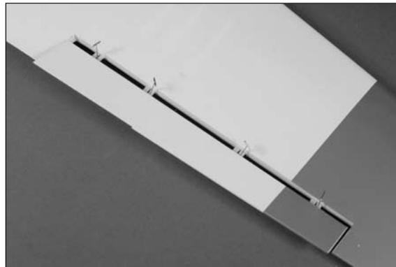
6. Remove the T-pins from the hinges. Make sure the aileron is pressed tightly against the wing panel to eliminate any hinge gap. Check that the ends of the aileron have an equal gap and are centered in the opening for the aileron in the wing panel.
