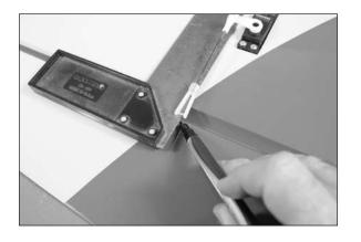
□□ 11. Move the aileron linkage out of the way. Position the control horn so it is centered on the line drawn in the previous step. With the front edge of the horn aligned with the taper of the hinge line, use a felt-tipped pen to mark the locations for the two mounting screws.
