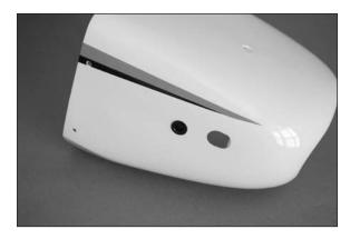
☐ 12. Trim the cowl to fit the muffler. The opening in the bottom of the cowl must be at least twice the size of the opening at the front to allow for air to pass over the engine for cooling. Guide the tubing for the fuel dot through the fitting in the cowl.
