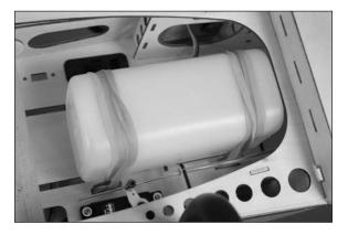
→ If you are installing a gas engine, simply route the vent line to the bottom of the fuselage.
