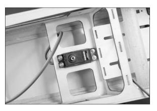
□□ 5. Prepare the elevator servo by installing the rubber grommets and brass eyelets. Secure a 24-inch (610mm) servo extension to the servo lead using dental floss so it doesn't accidentally become disconnected inside the fuselage.
