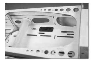
→ The location of the receiver battery is determined by your choice of engine and how the airframe balances. It may be necessary to relocate the battery to achieve the best balance for your model. The battery location shown may or may not be correct for your choice of power systems.
