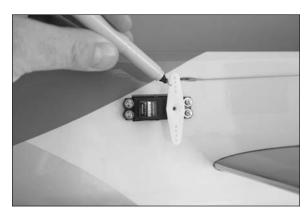
□□ 12. Assemble the elevator linkage as shown using a 2mm x 115mm pushrod, M2 ball link and a nylon clevis. Make sure to slide a piece of safety tubing on the clevis before threading it on the pushrod. Adjust the length of the pushrod so it measures 5.75 inches (147mm) as shown in the photo below.
