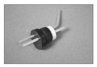
$\Box$  6. Slide the larger stopper plate over the tubing at the front. Start the M3 x 20 screw using a #1 Phillips screwdriver. The screw only needs to be in far enough to keep the large stopper plate from falling off. Slide the fuel tubing on the straight piece of aluminum tubing. The clunk will be placed on the opposite end of the fuel tubing.
