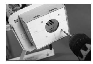
$\square$  4. Use a drill and 9/64-inch (3.5mm) drill bit to drill the hole for the throttle pushrod.
