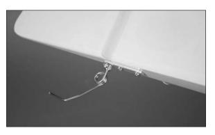
☐ 14. Place a drop of light machine oil on the tail wheel axle. Use two 2mm wheel collars to secure the 1.25-inch (30mm) tail wheel to the tail wheel wire. Use a #1 Phillips screwdriver to tighten the setscrews. Make sure the tail wheel can rotate freely when installed.
