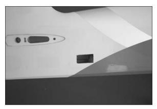
□□ 7. Route the lead for the elevator servo through the fuselage, under the formers. Fit the elevator servo in the opening with the output shaft facing toward the rear of the fuselage.
