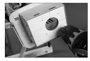
$\square$  3. Remove the template. Use a drill and 11/64-inch (4.5mm) drill bit to enlarge the holes in the firewall.
