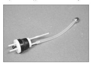
→ If you are assembling the fuel tank for use with a gas engine, you will need to use solder and a soldering iron to create a small barb for the fuel lines before they are installed. This is necessary as the tubing will need to be wired on to prevent it from sliding loose.
