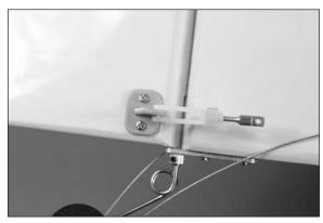
□□ 14. Remove the tape holding the cable to the fuselage. Slide a brass crimp on the cable, then pass the cable through the brass connector. The cable then goes back through the crimp. Do not tension the cable until instructed to do so.
