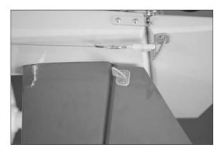
□□ 11. With the radio system on and the elevator servo centered, place the HD servo horn on the servo. The horn will be perpendicular to the servo centerline as shown. If not, remove the arm from the servo and rotate it 180 degrees and recheck the alignment. One position will be closer than the other, as the servo output shaft has an odd number of splines. Once aligned, mark the side of the servo horn facing toward the bottom of the fuselage, as it will need to be trimmed in the following steps.
