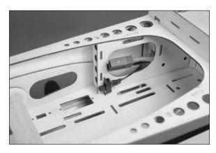
☐ 12. Secure the motor battery in the fuselage using hook and loop straps (not included). To keep the battery from sliding on the battery tray, use hook and loop tape (not included) between the battery and battery tray.
