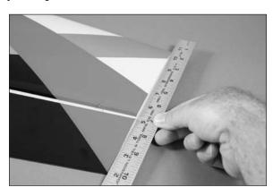
□□ 5b. (Side Force Generators) Position the aileron so it is set back 1/16-inch (1.5mm) from the wing tip. Use a straight edge at the wing tip to make sure the aileron is set back and can move freely without contacting the straight edge.
