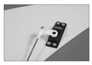
□□ 10. Use a square along the aileron hinge line to align the linkage perpendicular to the hinge line. Use a felt-tipped pen to mark the aileron where the center of the clevis is positioned.
