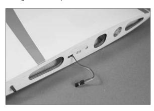
□□ 3. Place the servo in the opening with the output shaft of the servo facing toward the trailing edge of the wing. With the aileron servo centered in the opening, use a pencil to mark the locations for the four mounting screws. Remove the servo from the wing. Use a pin vise and 1/16-inch (1.5mm) drill bit to drill the holes for the mounting screws. Use care not to accidentally drill through the top of the wing.
