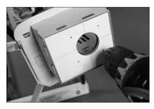
$\square$  6. Remove the template. Use a drill and 11/64-inch (4.5mm) drill bit to enlarge the holes in the firewall.
