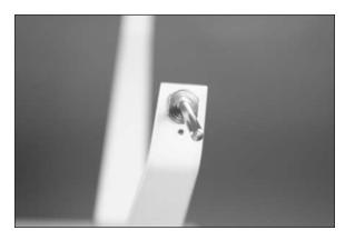
□□ 4. Prepare the axle by filing two 5/16-inch (8mm) wide sections on the axle. The first section is against the mounting flange of the axle, while the second section is the first 1/4-inch (6mm) of the axle as shown.
