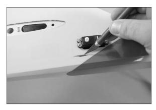
□□ 7. Insert the cable through the opening. Use a small piece of low-tack tape to secure the end of the cable so it doesn't fall out while maneuvering the fuselage. Make sure the cable is routed through the center of the formers.
