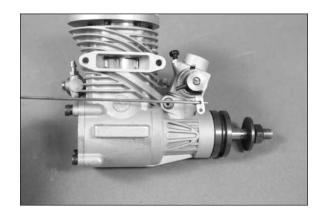
☐ 14. Reposition the engine between the mounting rails, guiding the pushrod into the pushrod tube. Secure the engine using four M3 x 25 socket head screws, eight M3 washers and four M3 lock nuts. Place the washers between the head of the screw and engine mounting lugs, as well as between the engine mount and M3 lock nuts. Tighten the hardware using a 2.5mm hex wrench and a 5.5mm nut driver.
