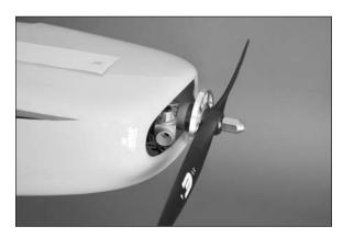
☐ 4. Position the cowl so the spinner is centered in the opening at the front of the cowl. Leave a gap of 3/32-inch (2mm) between the backplate and cowl so the backplate won't rub on the cowl. Use low-tack tape to secure the cowl to the fuselage.
