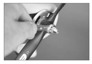
→ Do not use pliers or an adjustable wrench to tighten the propeller adapter. These tools will eventually round the edges of the nut, making it difficult to tighten or remove.
