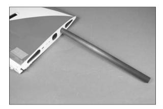
□□ 3. Slide the wing into position on the fuselage. Don't slide the wing tight against the fuselage at this time. Use plastic to prevent gluing the wing to the fuselage. Fit the wing root extension to the wing. Check the fit of the wing root extension by sliding the wing and extension tight against the fuselage. The outside edge will align between the wing and extension as shown.
