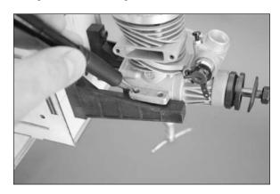
☐ 10. Remove the engine from the mount. Use a drill and 1/8-inch (3mm) drill bit to drill the holes for the engine mounting bolts.
