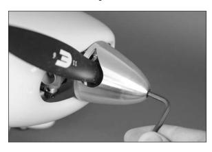
→ Make sure the propeller is centered in the openings so the spinner does not rub against the prop blades, which could potentially cause them to fail.
