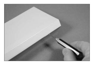
□□ 3. Prepare the four hinges by placing a T-pin in the center of each hinge. This will center the hinge when the aileron and wing are joined. Place the hinges in the hinge slots in the aileron. The T-pin will rest on the leading edge of the aileron as shown.
