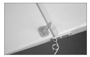
☐ 5. Repeat steps 2 through 4 to install the remaining control horn.
