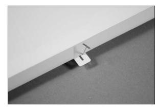
$\square \square$  4. Use the hinges to fit the aileron to the wing.
