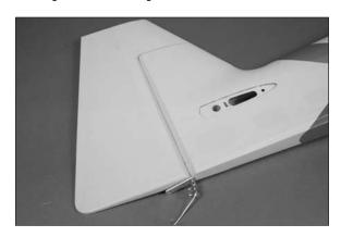
→ Do not glue the rudder hinges until instructed to do so.
