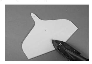
$\square \square$  2. Use a hobby knife and #11 blade to remove the covering to expose the two blind nuts at the wing tip.
