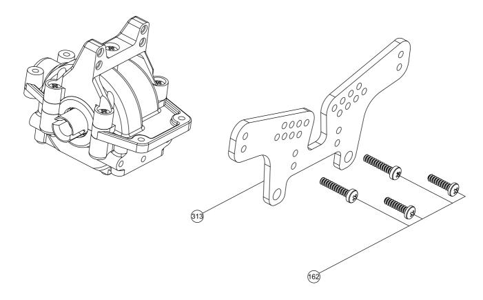
Fit the front shock tower and servo save system using screws as shown on the drawing.
