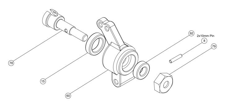
**Rear Hub Carrier Assembly:** The rear hubs on the Conqueror Rally are the same left and right. Push a 10x15x4 bearing into the inside of the hub and an 6x12x4 bearing into the outside of the hub. Slide a wheel axle through the bearings. Slide a wheel hub over the axle, lining up the holes in the axle and wheel hub. Push the 2mm pin through the hub and axle. Repeat for other hub.
