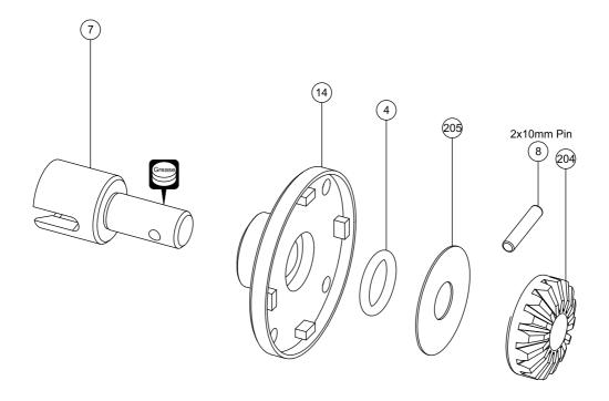
**Front/Rear Conical Gear:** Slide the bearing over the output shaft of the front/rear diff cap. Apply a light coat of grease to the male portion of the front/rear diff out drive and insert it through the diff cap. Apply a very light coat of grease to the o-ring, then slide it over the shaft of the out drive and seat it in the diff cap. Slide 1 shim behind each large bevel gear. Insert the pin through the hole in the shaft of the out drive. Check to make sure the out drive rotates freely.
