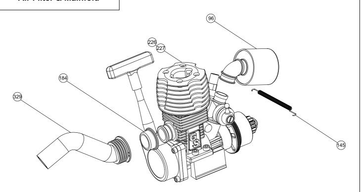
**Air Filter:** Push the air filter base onto the air filter adapter and secure with a small tie wrap. Apply a liberal amount of air filter oil (not included) to the air filter foam element and slide onto the air filter base. Attach and tighten the air filter end cap with a 3x6mm FHT screw. Wait until your radio settings are complete to attach and secure the air filter.
