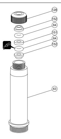
Apply a drop of GS Racing Pure Silicone Shock Oil to the o-rings. Place a shaft groove, followed by an o-ring, and one o-ring spacer, followed by another o-ring than place another shaft groove on the shock body. Tighten the lower cap for shock body.
