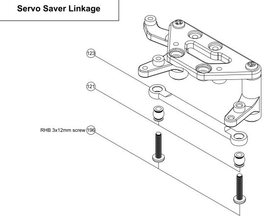
Snap the 5.8x6.3mm pivot ball studs into each end of the steering linkage. Slide the end of the arms into the steering mount (RD) and steering mount (L).
