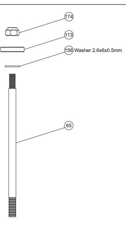
**Shock Body/Piston:** For the shock piston assembly, slide the 2.6mm washer over the stepped end of the shock shaft. Place the shock piston, over the shaft and washer. Tighten the piston in place using the 2.5mm lock nut. Repeat for the 3 other shock shafts.
