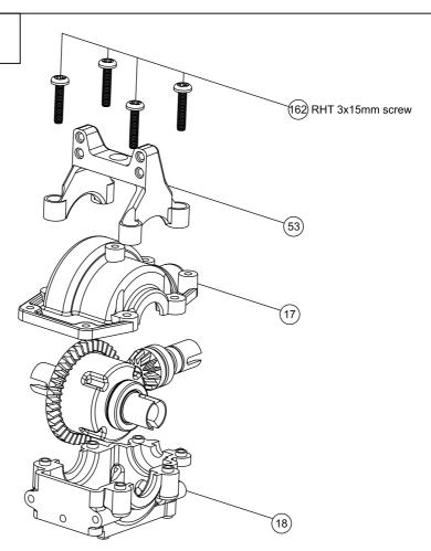
Fit the shock tower mount, gear box cap and gear box mount using 4pcs 3x15mm RHT screws at the same time on it.
