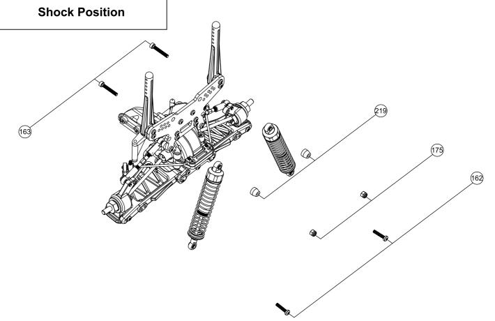
Rear Shocks: Attach the shocks to the shock tower and lower arms at the outside holes of the arms using 3x15 RHT screws.
