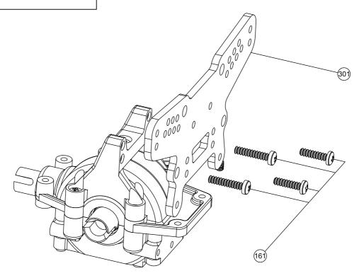
Fit the rear shock tower, rear end brace and Rear end brace mount using screws as shown on the drawing. And also fit the wing mount of exhaust pipe set using screws as shown on the drawing.
