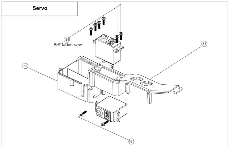
**Servos:** Attach throttle servo (shown at top of drawing) to radio tray using 3x12mm RHT screws. Attach the steering servo (shown at the bottom of the diagram) to radio tray posts. Do not over tighten any of the screws, only tighten until snug.
