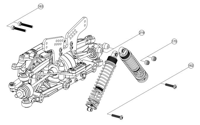
**Front Shocks:** Attach the shocks to the shock tower and lower arms at the upper holes of the arms using 3x15 RHT screws.
