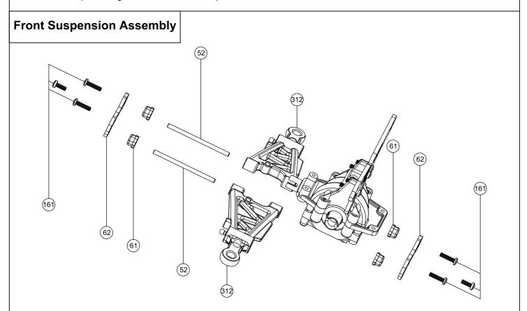
All Conqueror Rally are using non e-clip suspension system. Insert the toe-in plate inserts, note side up, into the front toe-in plate. Slide the hinge pins into the front toe-in plate and slide the lower arm assemblies over the hinge pins. Insert the front rear suspension mount inserts, note side out, into the front rear suspension mount. Slide the mount, with the inserts attached over the hinge pins.
