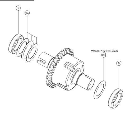
Slide washers(159) between the each diff out drive and the bearing.
