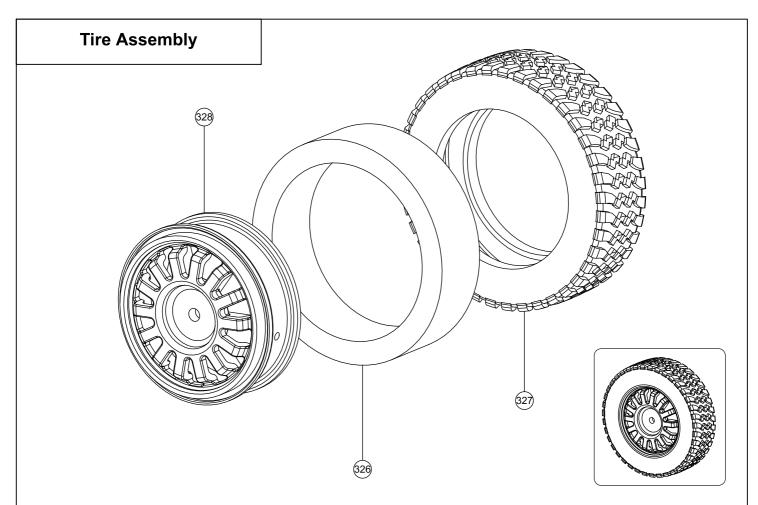
Clean contact area of the wheels and tires with rubbing alcohol or window cleaner before gluing!
