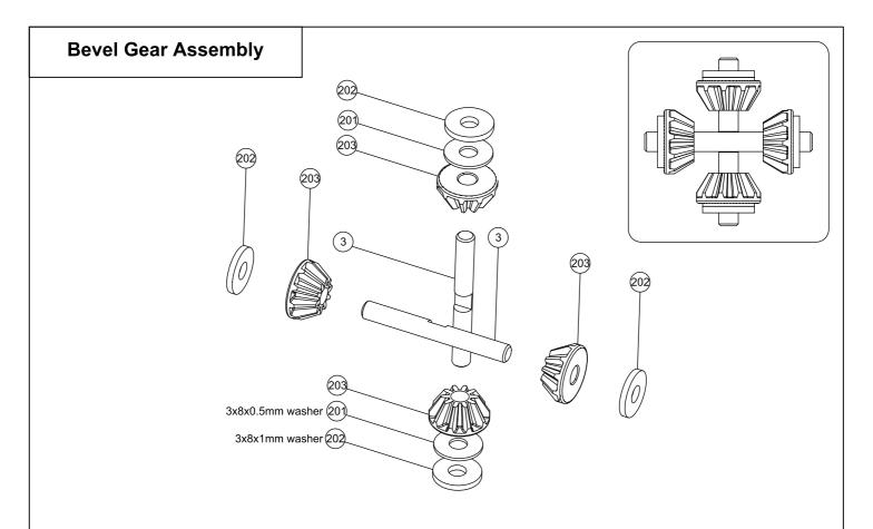
**Bevel Gear Assembly**: In this step you will build the small bevel gear assemblies for all 2 differentials. Slide 2 small bevel gears, small sides toward each other, over the shaft. Repeat on second shaft. Place one shaft assembly over the other, the flat portions locking into each other. The shims behind the gears should be flush with the ends of the shafts.
