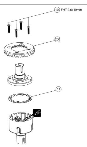
Attach the 39T Ring gear assembly using 2.6x10mm FHT screws. Tighten the screws in a cross pattern until firmly sunk, do not over tighten!
