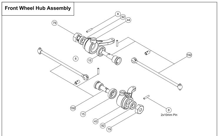
Steering Knuckles: Push a 10x15x4 bearing into the inside of the hub and a 6x12x4 bearing into the outside of the hub. Slide a CVD's axle through the bearings. Slide a wheel hub over the axle, lining up the holes in the axle and wheel hub. Push the 2mm pin through the hub and axle. Repeat for other hub.
