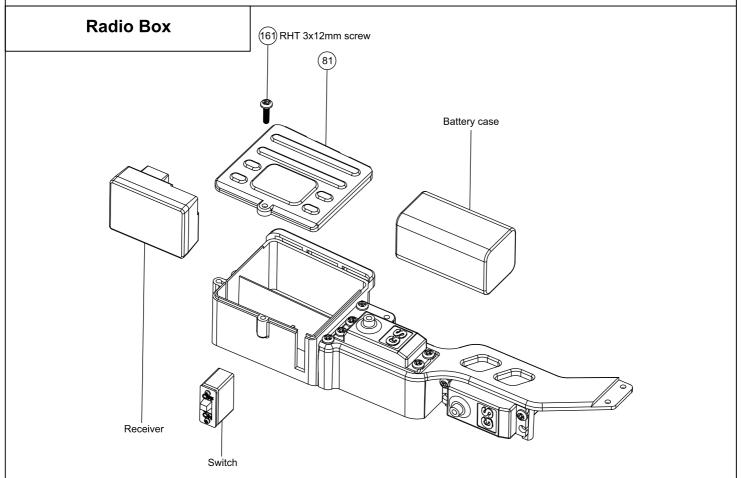
**Radio Box:** Mount the on/off switch into radio box bottom with the "on" side facing toward the ground. You may install the silicone switch cover included in your kit over the switch before installation.
