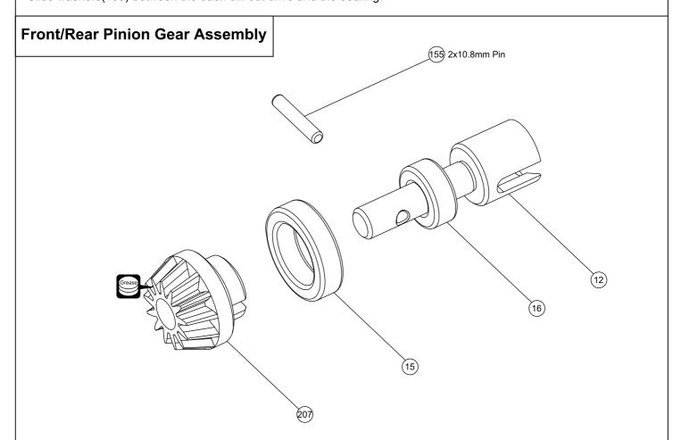
Insert the pin through the hole in the shaft of the pinion gear out drive.
