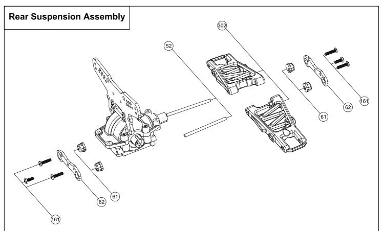
The Conqueror Rally is using non e-clip suspension system. Insert the anti-squat inserts, note side up, into the anti-squat mount. Slide the hinge pins into the anti-squat mount and slide the lower arm assemblies over the hinge pins. Insert the rear suspension mount inserts, note side out, into the rear suspension mount. Slide the mount, with the inserts attached over the hinge pins.
