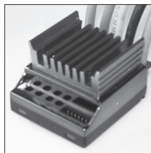
LRP SPX Competition StockSpec with mounted heatsink.
