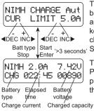
This program is for charging of NiCd/NiMH batteries associated with R/C models applications. You can press START/ENTER key to make it blink and then INC or DEC to change the parameter value. Press START/ENTER key to store the value.
