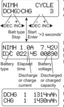
You can set up sequence on the left and the number of cycles on the right. Range of the cycle number is 1-5.
