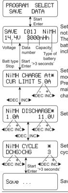
Setting of the parameter in the screen will not affect the charge and discharge process. They just present the specification of the battery. The example is NiMH battery pack, including 12 cells, the capacity is 3000m Ah.
