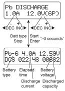
Set up the charge current on the left and nominal voltage on the right. Range of discharge current is 0.1-1.0A, the voltage should match the battery being charged. Press START/ENTER key for more than 3 seconds to start charging.
