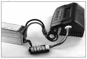
The main battery leads must be connected along with the balance lead connector as shown before charging your battery .
