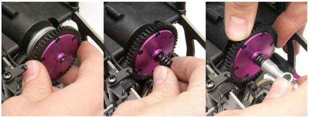
Fit the new spur gear and replace the washer, spring and nut
