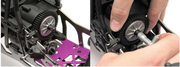
Undo the nut that holds on the slipper clutch
