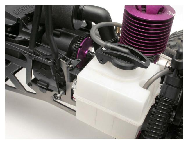
Replace the fuel tank, fuel lines and the R clips and you are good to go!
