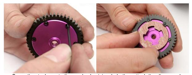
Screw the steel gear to the purple aluminium hub, then attach the slipper pad
