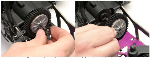
Remove the spring, washer and the slipper clutch parts
