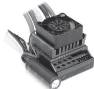
Mount the power-capacitor in a position where it is protected in the event of a crash. The best place is right next to the speed-control (see picture). Secure it with doublesided
