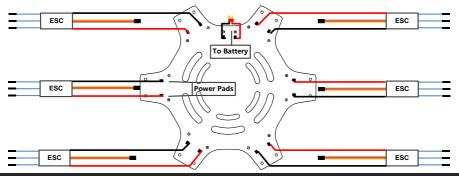
Please solder ESCs to bottom board as the up figure shows. Use any insulating method at all soldering spots.
