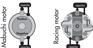
**ONLY FOR BRUSHED MOTORS!** Motors with no capacitors or not enough capacitors may interfere with the speed-control. To avoid this, solder the supplied capacitors to your motor (see picture).
