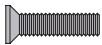
Z449 Flat Head Screw M2.5x12mm Senkkopfschraube M2.5x12mm Vis tête fraisee M2.5x12mm Tornillo avellanado M2,5x12mm
