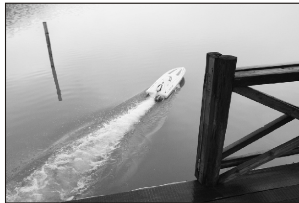
16. It is required and suggested to put the boat in water as soon as engine starts, if you tune the engine too long or too high then engine will be overheated. You will have to let engine water cooled by running the boat.
