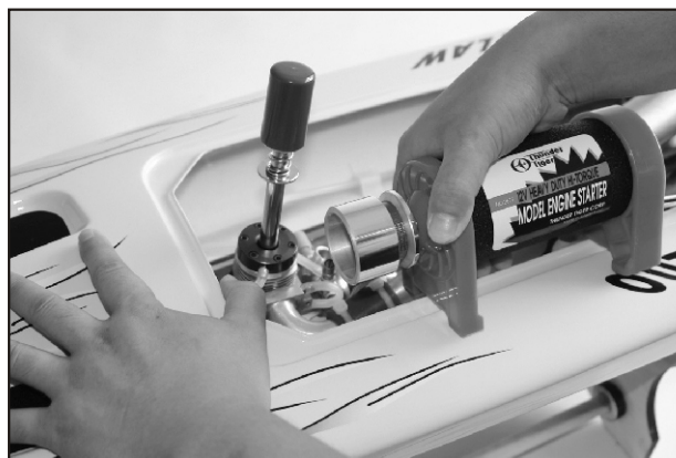
14. Screw in the glow plug then start the engine. Suggest to use high voltage 18-24v starter for easy starting, if a normal 12V starter is used then unscrew the glow plug by 1/2 turn for less compression is required or it is hard to start. You will need one assistant to help you start the engine. Hint: You may wisely to turn on starter first then pull the belt, this is to let starter has a initial speed for easy rotating. If belt is pulled before turning on the starter then starter may be not torque enough to rotate.
