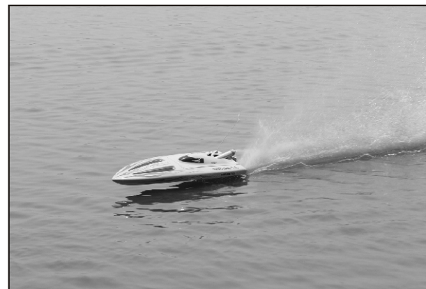
17. It is required to run the boat at least middle speed around 20 mph/ 32 kmp so it is fast enough to draw the water from rudder to engine and pipe. Always check if there is water out from the port. No water goes out the engine will overheat very soon.
