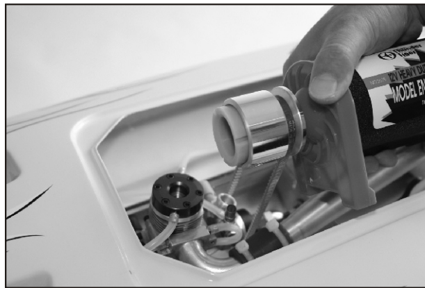
13. You may do this way several times to clean the engine before Break-In. Note: Keep away from the spray out fuel, use your hand to feel fuel spray until it is foggy.
