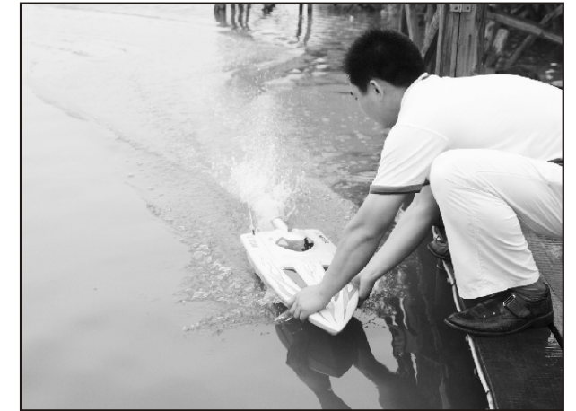
21. After cruising, come back to the pier then stop the engine by pushing the trigger. Always take great care and away from the hot pipe and sharp water fin. Check all screws again, make sure they are tightened.
