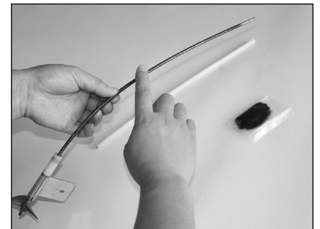
22. Lubricate the drive shaft is important. You will need two 17mm wrench to loosen the coupler. Take out the shaft by unscrewing the strut from the mount. Suggest to exam the shaft every 5 runs, clean and apply new grease is required. Replace new tube and shaft if they are worn out.
