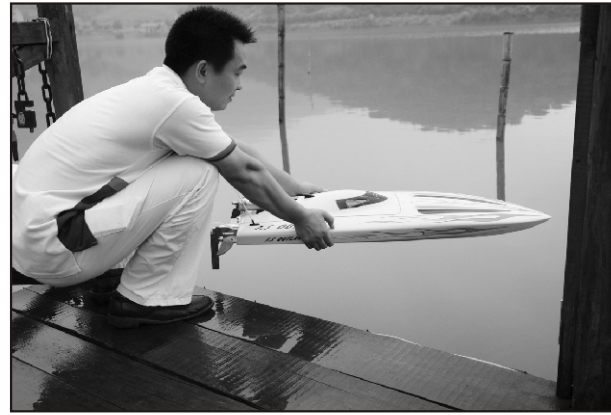
15. Place the boat in water to break-in the engine or engine will overheat and be damaged. As soon as the engine starts, trigger the throttle and make sure the engine rotates counterclockwise, remove the glow starter, well position the belt in the notch then put on the hatch cover. Next place the boat in the water and go.
