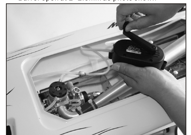
11. Unplug the fuel line from carb then pump the fuel to tank, 15% of Nitro is recommended. Of course the higher percentage of Nitro, the more of the power. However, high nitro means higher price and also will decrease the life of engine.
