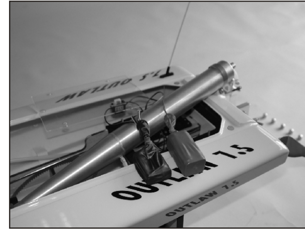
7. Use balloon to well wrap the receiver and battery holder, next seal the opening with the small rubber band. This will help to resist from the water or humidity.
