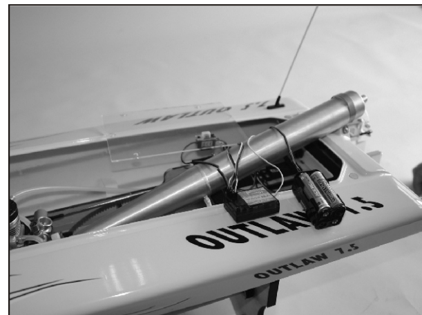
6. Install 4 dry cells or rechargeable battery in the battery holder. Change to 3600mAh 4.8V NiMH battery pack is recommended. Insert the antenna tube in the antenna mount.
