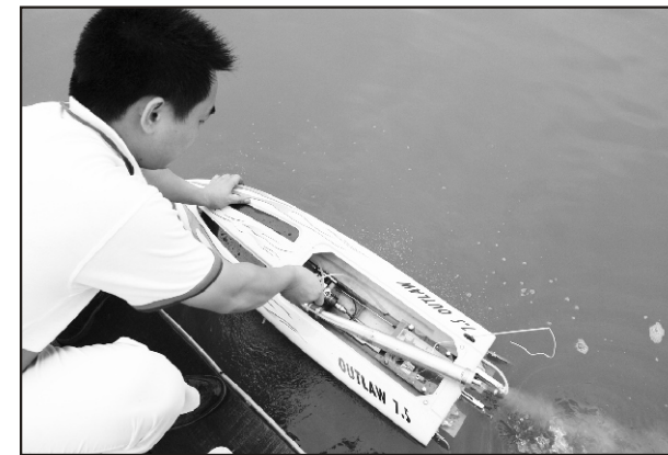
19. If boat is too slow then come back to the pier and adjust the main needle. Suggest to tune 1/4 turn each time until you feel it is faster. Once you feel it is getting higher but not the peak then tune 1/8 or 1/16 turn in each time for peak performance.
