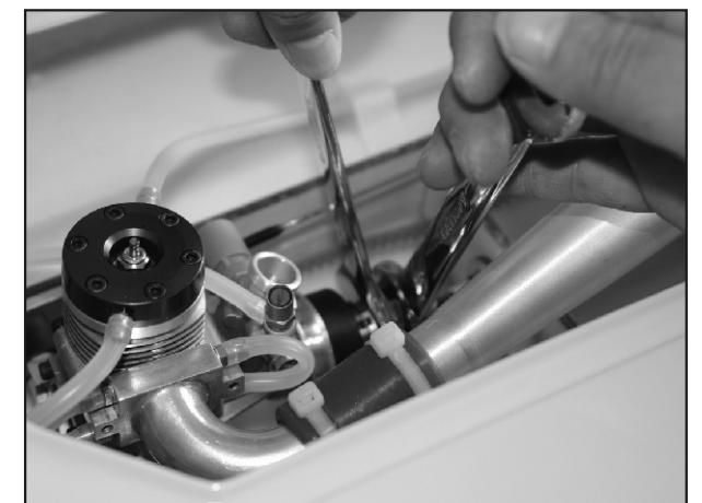
21. After cruising, come back to the pier then stop the engine by pushing the trigger. Always take great care and away from the hot pipe and sharp water fin. Check all screws again, make sure they are tightened.
