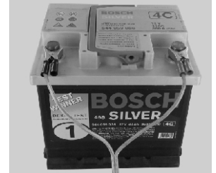
Using terminal clip attaching to car battery
