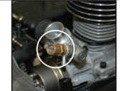
High Speed Mixture: 2 3/4 turns out Clockwise = Leaner Counterclockwise = Richer
