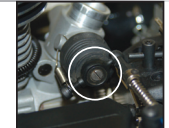
Low Speed Mixture: 6 1/2 turns out at full throttle Clockwise = Leaner Counterclockwise = Richer
