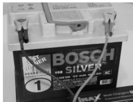
Using terminal clip attaching to car battery
